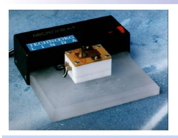
The MicroHeat is a small, compact hot pate which allows an easy method for mounting 3mm TEM specimens prior to grinding and polishing or ion beam milling. During the specimen preparation process it is critical to mount the specimen properly, and the unique size of the MicroHeat allows observation of the mounted specimen with a stereo microscope. This allows high quality specimens to be prepared with accuracy.
